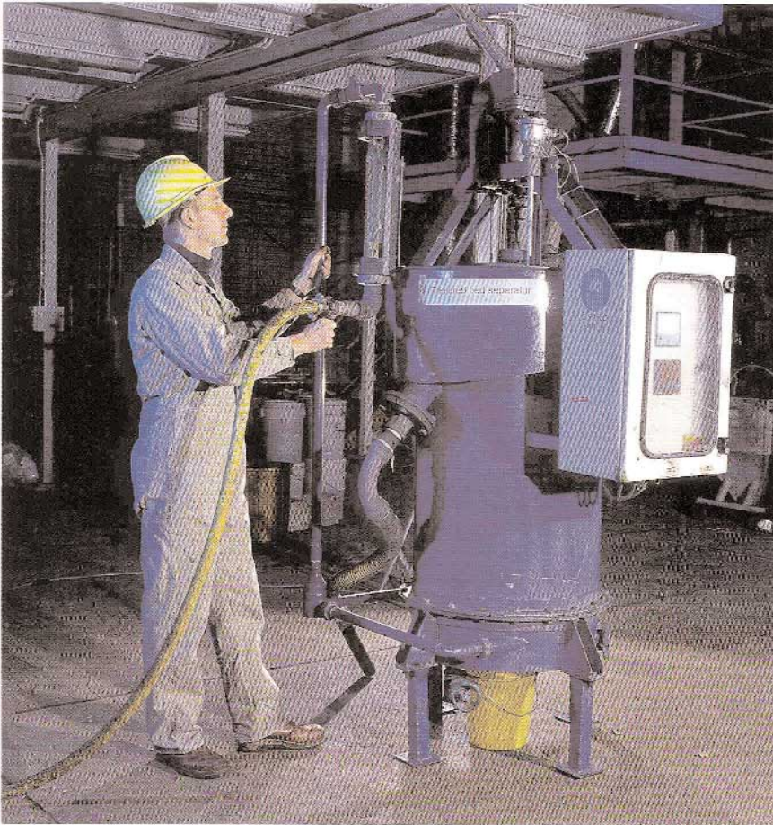
Fig. 5: Pilot-scale 0.6 m teetered bed separator at CSIRO
